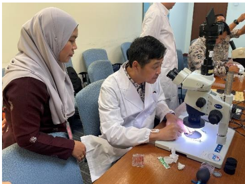
Adjustment of samples using a stereo microscope
